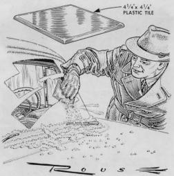
For scraping snow or frost from the windshield, stow a plastic tile in the glove compartment. The tile has four sharp edges that will quickly clear the glass without scratching it, and, being flexible, the tile will bend to fit the curves.
