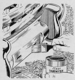
Rust often starts unnoticed where the bumper is covered by the license plate, then spreads rapidly outward. You can prevent this by protecting the chrome in that area with a coat of clear varnish before you bolt on the plates.
