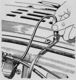
Windshield washer won't squirt? First, be sure there's water in the reservoir. Then disconnect the tube at the washer nozzle and slip it over the discharge end. Operate the washer a few times to reverse-flush the nozzle and clear it.
