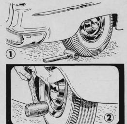
A rubber mallet is useful in two ways when you change a wheel: Place it under one of the other wheels as a safety chock to keep the car from rolling; when the job is done, pull it out by the handle to use it for driving on the hubcap.
