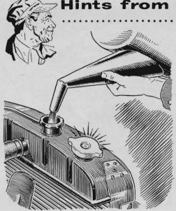
Your radiator cap is less likely to be left unnoticed after the coolant has been checked if you paint it bright yellow. Paint the underside, too (but not the pressure seal), to make it conspicuous even if it is set aside upside down.
