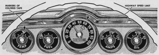
TEMPERATURE GAUGE. Place marker on glass in line with needle after stabilizing engine's temperature by driving the car for at least half an hour. FUEL GAUGE. Run engine until fuel in tank is exhausted. Then pour in three gallons and mark position of needle so you'll know your gallon reserve.
