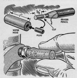
Protective caps, quickly made from windshield-wiper hose, will keep grease fittings clean and make them easy to find. Cut the hose into 1" pieces and close one end with plugs cut from an eraser stick. Clean the fittings before you cap them.
