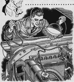
Make a trouble lamp that really illuminates the work area. Use an old two-beam headlight in which one filament has burned out. Solder wires about 12 feet long to the good terminals of the bulb and attach battery clips to the wire ends.
