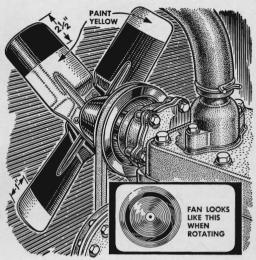
A rotating fan will show up clearly as a yellow disk with a black ring when part of each blade is painted yellow for safety, as shown above. To avoid splashing, use a fast-drying paint and let it dry thoroughly before starting the engine.
