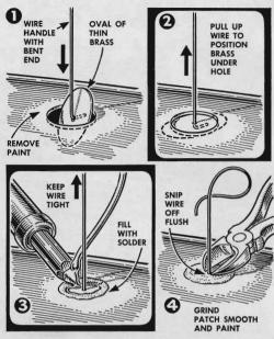
**To fill a screw hole** after removing an accessory, back it up with an oval of brass held in place with a wire. Flow solder over it to build up the surface and snip off the wire when the solder sets. Grind the patch flush and paint to match.
