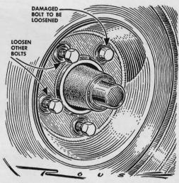
When a wrench won't grip the head of a damaged wheel lug, you can sometimes jar it loose. With the car jacked up, loosen the other lugs. Then lower the car and rock it back and forth to make the wheel shift slightly, causing the lug to turn.
