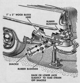
Worn spring bushings can be replaced without effort. Jack up the chassis until there is room for a block of wood between the spring and hanger eyes. Then lower the chassis. With tension off the spring, the shackle can be removed easily.
