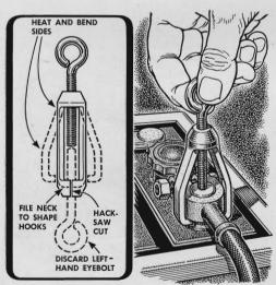
A safe battery-terminal puller can be made from a turnbuckle. Discard the lefthand evebolt and hacksaw the threaded end down the middle. Spread the sides and file off enough from the split end to make hooks that fit under the cable clamps.
