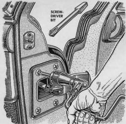
For that extra leverage needed to loosen the adjusting screws on door hinges without damaging their heads, try a carpenter's brace. Screwdriver bits with shanks to fit the brace can be purchased for both Phillips-head and slotted screws.
