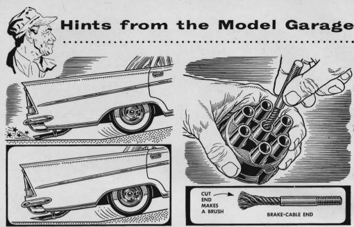
A tailpipe that scrapes as you enter or leave a steep driveway can be cut without shortening it. Hacksaw a piece from the bottom of the pipe at a long angle. You gain road clearance, yet the overhang keeps the bumper free of exhaust stains.
