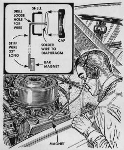
**To pinpoint engine noises,** use a stethoscope made from a radio earphone. Solder a stiff wire to the diaphragm, and the earphone's magnet to the wire's other end. Touch the magnet to different parts of the engine to listen and trace noises.
