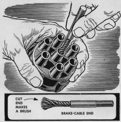
Corrosion can be cleaned from inside distributor-cap terminals with a wire brush made from a discarded hand-brake cable. Cut the cable near its end and use its adjusting rod as a handle. Unravel a few strands, insert in the terminals, and twist.
