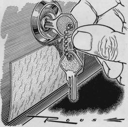
The noise of keys jangling against the dash can be silenced by cementing a small square of leather to the metal below the ignition switch. Rubber cement will hold it without damaging the finish. Colored leather can be bought at craft shops.
