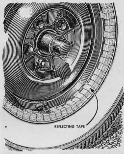
**Short strips of reflecting tape** placed side by side around wheel rims serve two purposes: They reflect an oncoming car's headlights when you drive out of a side street and they eliminate any occasional tendency for the wheel covers to creak.
