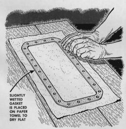
A cork gasket that has shrunk can sometimes be restored to its original size by dipping in water and laying it flat long enough to absorb the moisture and swell. Don't soak it for a long period of time, as it might come apart or crumble.
