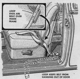
**Opened seat belts** can be kept from dangling out the door by threading the two outer belts through loops bent from heavy copper wire. Insert the loops in holes punched in the seat frame with an ice pick and bend the ends over.
