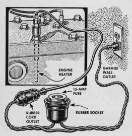
**Protect an engine heater** by plugging it into a short, fused extension line. Use No. 12 or 14 wire with a plug at one end and a rubber outlet at the other. Cut one leg of the cord and install a rubber socket to hold a 15-amp house fuse.
