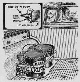
**Cargo can be secured** in a station wagon by fastening several sets of rifle-sling swivels to the sides and floor of the vehicle with sheet-metal screws. Used with several random lengths of web strap, almost anything can be safely tied down.
