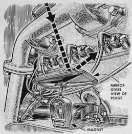
**To help you see** beneath the manifolds when installing plugs in new V-8s, fasten an old rear-view mirror to a husky magnet. Place it on the frame with the mirror aimed at the plug openings and you can work without feeling your way.
