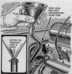
A hose attached to a funnel will help get automatic-transmission fluid to a filler tube that is close to the car's firewall. Use hose that will fit in the filler tube and slip it over the funnel's neck. A cotter pin will hold the hose in place.
