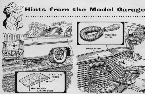
A pair of rounded wood blocks anchored to a sloping driveway will keep a car from rolling away. The blocks should be gently rounded so they are easy to run over, yet at the same time just steep enough to hold the car when it is parked.
