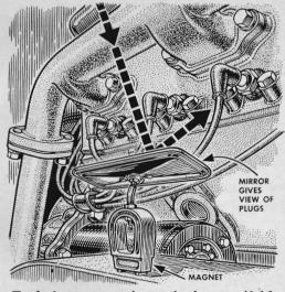
**To help you see** beneath the manifolds when installing plugs in new V-8s, fasten an old rear-view mirror to a husky magnet. Place it on the frame with the mirror aimed at the plug openings and you can work without feeling your way.
