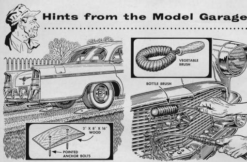
A pair of rounded wood blocks anchored to a sloping driveway will keep a car from rolling away. The blocks should be gently rounded so they are easy to run over, yet at the same time just steep enough to hold the car when it is parked.
