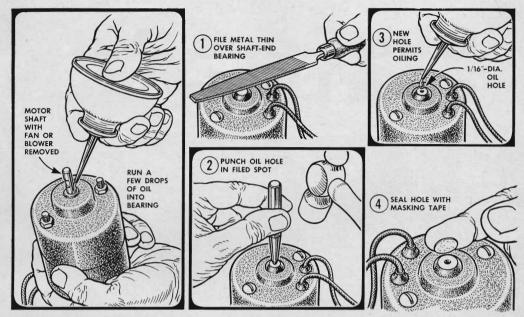
**Small heater and electric-wiper motors** are often neglected because they must be taken apart to be oiled. A drop in efficiency results. Simplify the problem by providing an oil hole in the sealed housing-end. File the metal thin but not
