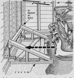
A tapered car-stop of two-by-fours built against the garage wall serves a double purpose: It prevents accidentally ramming the wall; and as the bumper rides up on it, the car's weight is off the front springs, postponing front-end sag.
