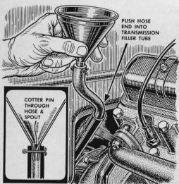
A hose attached to a funnel will help get automatic-transmission fluid to a filler tube that is close to the car's firewall. Use hose that will fit in the filler tube and slip it over the funnel's neck. A cotter pin will hold the hose in place.
