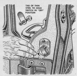
**Sitting in a drive-in** on a warm night, you can keep the car doors open without burning the dome and courtesy lights. Install metal tabs on the door switches and swing them over the switch buttons to hold them in the "off" position.
