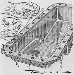
Tie a cork gasket in place with light sewing thread to keep it from slipping out of position during installation. The thread needn't be removed, as it won't interfere with the seal or the insertion of bolts. For neatness, trim off the free ends.
