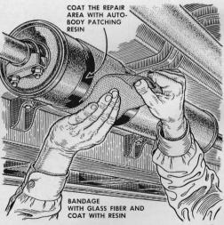
A permanent muffler repair can be made with a glass-fiber body-patching kit. Wire-brush the area around the damaged part and apply a coat of liquid resin. Then wrap a strip of glass-fiber cloth around it and saturate it with resin.
