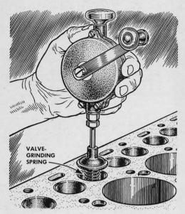
To avoid scoring valve seats when grinding-in valves, always install a lifter under the valve before beginning work. It is a constant reminder to ease up on the grinding pressure and lift the valve frequently to redistribute the compound.
