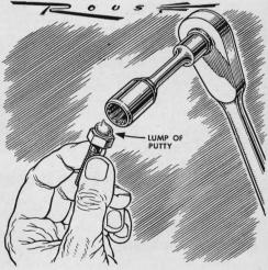
**Stick bolts, nuts or cap screws** in a socket wrench with a small lump of putty to hold them while you start them in hard-to-reach places. Leave the sticky stuff in the socket for the next hard job; it won't interfere with normal use.
