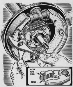
**Brake-shoe retracting springs** can be installed with ordinary pliers fitted with a flathead nail. Hook the free end of the spring on the nail and stretch it across to the opposite shoe by squeezing the pliers against the brake lining.
