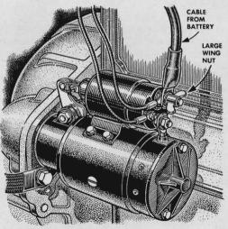
tip: Fasten the battery cable to its terminal on the starter solenoid or junction box with a wing nut, as above, in place of the regular hex nut. You can now disconnect the battery in seconds, without tools, to prevent a fire in case of a short.
