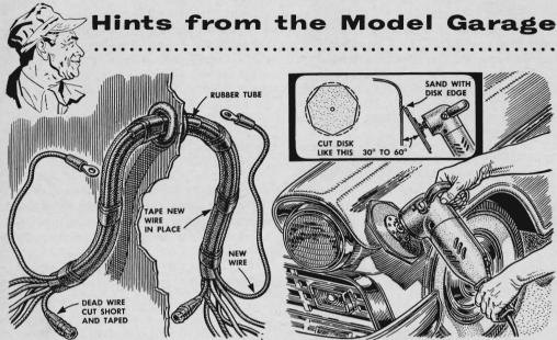
To replace a bad wire in a harness, cut both ends out of service and tape them over. Install a new wire of the same gauge by running it along the outside of the harness and taping it in place at intervals. Use rubber tubing at chafe spots. Reach into the deep spots when you clean metal for filling with lead. Worn abrasive disks, cut into polygonal shapes, will flex themselves into the recesses. Bring the tips of the spinning disk into light contact with the metal surface.
