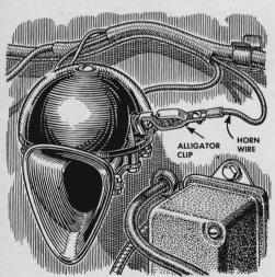
Disconnecting electrical wires fast is sometimes necessary. By having the foresight to install alligator clips on horn wires (above, left), you can yank them off immediately if the horn should stick and sound off continuously. A second
