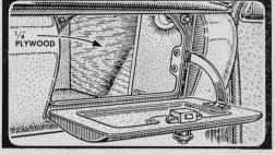
A plywood shelf or vertical partition installed in the glove compartment keeps road maps neat and separate from other articles. Fasten the wood dividers with thumbtacks driven through the fiber sides or bottom of the compartment.
