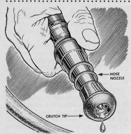
A hose nozzle can't scratch or chip your car's finish if you cover its end with a rubber crutch tip. Cut a %" hole in the crutch tip to let the water through. Center this hole so that it won't interfere with the fine-spray adjustment.
