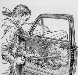
Freshen the faded interior of an older car by spraying it with fabric dye dissolved in hot water. Use a deeper shade of the original color and saturate the material. Masking isn't necessary as the dye can be wiped off metal, glass and paint.
