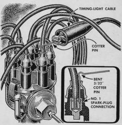
**Hook up a timing light** quickly with a bent cotter pin. One leg of the pin slips into the distributor cap's No. 1 spark-plug socket; the timing-light cable clamps on the other. The distributor is often easier to reach than the plug.
