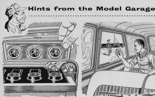
Hold a mirror over the cell openings of your car battery to see if the electrolyte levels are high enough. With vent plugs off, the liquid inside shows up clearly, saving you, with some models, an uncomfortable stretch under the bood
