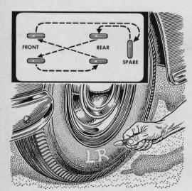
Switching tires can be simplified if you first mark their positions with a crayon (LR for left rear, for example). Then you can check later to see if they've been rotated properly (see sketch). Crayon won't come off during handling.
