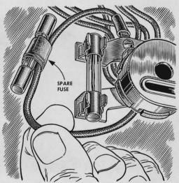
Tape a spare fuse on one of the wires leading to each fuse clip and it will always be handy when needed. But make sure the amperage of your spare matches that of the fuse to be replaced; amperage varies from place to place on a car.
