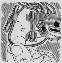
Tape a spare fuse on one of the wires leading to each fuse clip and it will always be handy when needed. But make sure the amperage of your spare matches that of the fuse to be replaced; amperage varies from place to place on a car.
