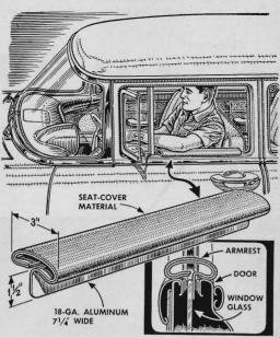
An armrest that fits over the window sill lets the driver rest his arm during long trips without burning it on hot car metal. Woven seat-cover material is cemented to a piece of aluminum shaped to slip between door and window glass.
