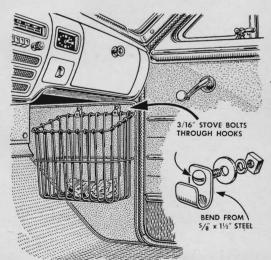
A litter container stores family trash until it can be emptied at a service station or at home—instead of on the highway. A bicycle basket hangs from hooks bolted to a panel under the dash and is easily removed and replaced.
