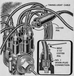
**Hook up a timing light** quickly with a bent cotter pin. One leg of the pin slips into the distributor cap's No. 1 spark-plug socket; the timing-light cable clamps on the other. The distributor is often easier to reach than the plug.
