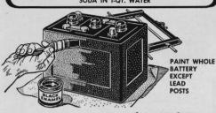
**Stop tiny current leaks** that steal power from your battery. Take it out of the car and wash off the current-conducting dirt with baking soda and water. When dry, paint the battery case, cell tops and hold-down bracket. Scrape the terminals and cable lugs clean for good contact and coat them with petroleum jelly.
