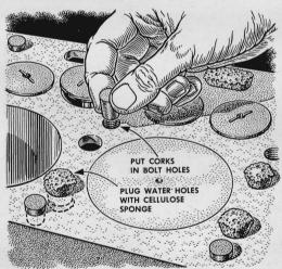
When working on an engine block with the cylinder head removed, plug the blind stud holes and water passages with corks or pieces of cellulose sponge to keep them free of carbon scrapings, valvegrinding compound and other loose dirt.
