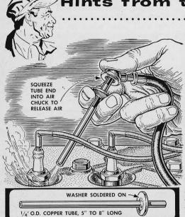
Use this blow gun to get dirt out of spark-plug recesses or to clean parts. It's inserted into a filling-station air-hose chuck, and, when pressed in, directs the blast of air where needed. A washer soldered to the tube serves as a trigger.
