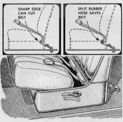
Protect safety belts from chafing on the sharp edge of a metal seat frame, or they may cut through under strain. Slit short lengths of heater hose and force them over the metal edge where the belts come through the seat.
