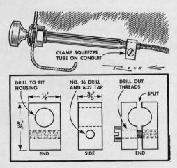
A flexible cable that's pulled loose because of too much yanking can be repaired with a clamp made from a block of steel. Machine as shown and tighten it around the housing neck to squeeze the metal tight on the flexible section.
