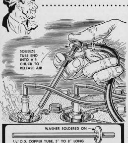
**Use this blow gun** to get dirt out of spark-plug recesses or to clean parts. It's inserted into a filling-station air-hose chuck, and, when pressed in, directs the blast of air where needed. A washer soldered to the tube serves as a trigger.
