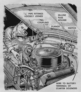
An under-hood lamp on swiveling pipe fittings puts light where you need it. Connect several feet of wire to a license-plate or map light and thread it through the fittings before loosely screwing them together. Bolt the unit to the fire wall.
