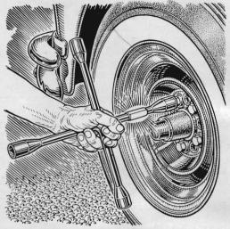
A strip of reflective tape wrapped around one shank of a four-way lug wrench saves fumbling for the right socket when changing a tire. Little disks of the tape stuck on the bolt heads may keep them from being lost if you get a flat at night.
