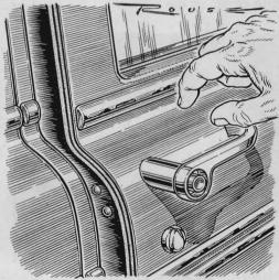
Opening the doors slightly when you put your car in the garage after being out in the rain can add years to the life of the car's body. This hastens drying at critical areas such as door bottoms, which are usually the first to rust.
