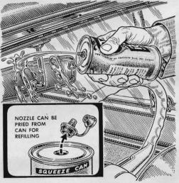
To clear your windshield quickly of slush and muddy road spray raised by the cars ahead of you, squirt some water on the glass while operating the wipers. Store the water in one of the new squeeze cans used for liquid detergent.
