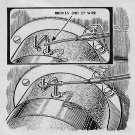
A terminal lug makes a neat repair where the eye of a flexible control cable has broken off. Select a lug with a hole the diameter of the eye it will replace. Tin the end of the control wire or cable, slip on the lug and solder it in place.
