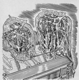
When washing or degreasing an engine, cover the carburetor, coil and distributor with plastic food-saver bags to keep them dry. After the washing, remove the covers and the engine should start easily, or at most after drying only the spark plugs.
