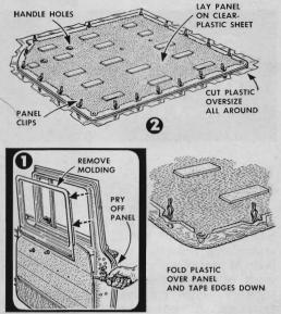
Keep the new look in your car's interior by covering the cowl and door panels with sheets of clear plastic. Pry off the panels and cut the plastic to fit with an inch overlapping all around. Fold the edges over and secure them with tape.
