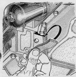
Cement a piece of felt over the openings that you'll find on some Chrysler-built cars between the rear of the oil pan and the left and right sides of the front face of the clutch bell housing. This keeps dirt out of the clutch assembly.
