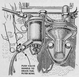
Quicker draining of fuel sediment can be provided in some cars and tractors by fitting on an airplane-type filter bowl in place of the regular glass bowl. These bowls have a drain valve at the bottom, which makes it unnecessary to remove the bowl itself. They are made in two diameters for light-plane fuel lines.
