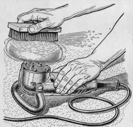
Fleece polishing pad gummed up with rubbing compound and polish? Put the buffer on the floor and turn it on, holding with one hand. With the other put a new wire brush gently against the fleece. This combs it out as clean as new.
