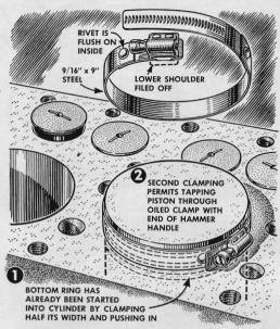
A piston-ring compressor can be improvised at little cost from a worm-gear hose clamp. File off one shoulder from the screw housing, hacksaw the gear band from the gear housing and rivet a strip of steel 9/16" wide and 9" long between them. Use the compressor as shown, first to compress one ring, then those above.
