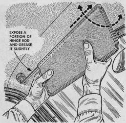
Up-and-down movement of a sun visor can be made easier on some cars by pulling it about halfway off the hinge rod with a twisting motion and applying just a touch of petroleum jelly. Don't pull it too far or apply too much jelly-you may loosen the visor too much.
