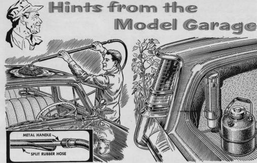
Protect the car finish if you use a moptype washer like this. Slit a piece of rubber garden hose lengthwise and slip it over the handle. In cold weather the hose will also keep your hands warmer.
