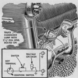
You can have back-up lights-practically in a jiffy. Buy a pair of chrome-plated truck clearance lights with clear lenses. They come complete with mounting brackets and are easily bolted in place. Wire in parallel. Control with a manually operated switch on the dash.
