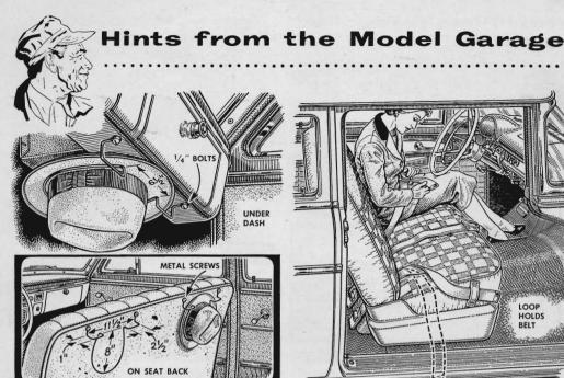
Your best hat won't get sat on if you stow it out of the way in a holder. Coathanger wire will do for back-of-seat holders, but hard No. 9 wire should be used under the dash to support the hat.
