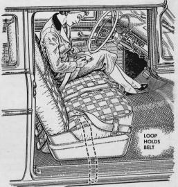
Keep safety belts from dropping out of the car by tucking the ends of the outer straps into loops stitched to the ends of the seat. The belts will stay cleaner, and won't get pinched by the car door.
