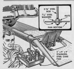
A hook-on tray hung within reaching distance will save fumbling for tools or parts while working under a car. The tray shown is kept stocked with wrenches and extra fittings for a lube job, saving the garageman many steps. On a repair job, the tray could hold small parts.
