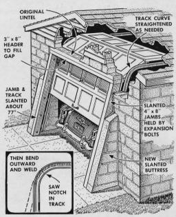
You can add footage to a garage that has the type of door shown. Remove the door jambs, notch the track where it curves and bend it out so that the door clears the car's bumper. Add an extra header to close the gap at the top of the door and reset the jambs to suit the track. Finish with slanted buttresses to match garage.
