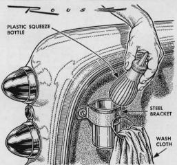
**Stow a plastic squeeze bottle** in a tin can screwed to the side of your car's trunk. Filled with windshield cleaner, it is convenient for keeping windows clear on a trip. In winter, fill the bottle with a defrosting solution to remove sleet.
