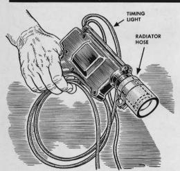
A short piece of radiator hose clamped over the lens end of a timing light will protect the light from being shattered if dropped or accidentally touched against a rotating fan blade. Paint the inside of the hose white to help throw light.
