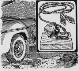
A compact trouble light can be assembled quickly using a truck clearance light, 15 feet of wire and a pair of battery clips. Bend the bracket to aim the lamp upward and screw it to a small block of wood. Having no batteries of its own, it won't be dead when you need it.
