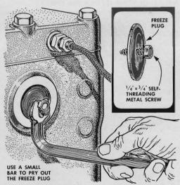
If a freeze plug leaks, tapping with a hammer will usually seal it. When this doesn't work, one mechanic drills a small hole in the center of the plug, turns in a metal screw about four turns, pries out the plug and drives in a new one.
