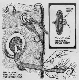
If a freeze plug leaks, tapping with a hammer will usually seal it. When this doesn't work, one mechanic drills a small hole in the center of the plug, turns in a metal screw about four turns, pries out the plug and drives in a new one.
