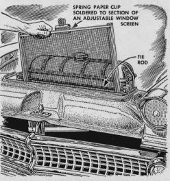
**During the bug season** one motorist keeps insects from plugging his radiator by slipping a section of an adjustable window screen into the opening behind the grille. A clip soldered to the screen rim holds it to the radiator tie rod.
