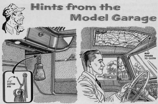
A cotter-pin hook like this will keep a whisk broom handy for sweeping out the car. Bend up one arm of the pin as shown. Then slip it over the side panel or through a hole punched in the panel.
