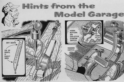
It's easier to check the oil in a warm engine containing light oil if you make a series of dents along the dipstick with a center punch. Oil held in the dents will be easily visible even when it's difficult to see any oil on the stick.
