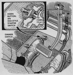
That idle left foot always bothers a veteran driver when he first drives a car that lacks a clutch pedal. Here's one man's solution-an auxiliary horn button on the floor. The switch is a singlepole, single-throw, normally-off job.
