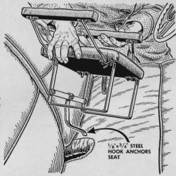
Anchoring a child's seat is a simple matter in cars with a center hole between the front seats. Bolt on a steel hook like this. Swing the hook in an arc through the hole to engage the seat securely, giving the child a safer ride.
