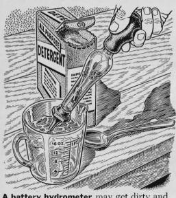
A battery hydrometer may get dirty and milky inside after long use. To clean, dissolve a tablespoon of detergent in a pint of warm water. Suck the solution into the hydrometer and let it stand for a half hour. Then rinse with clean water.
