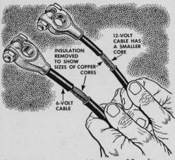
A 6-volt battery cable on a 12-volt car works fine, but don't try it the other way around or you'll get sluggish action. The reason? To save copper, manufacturers make 12-volt cores smaller since they must carry only half the amperage to produce the same wattage (volts × amps).
