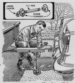
A removable caster like this will keep a small trailer level when it's unhitched —and make it easier to shove around. Bolt the flange to the underside of the tongue. Carry the rest of the caster unit in the trailer or tow car. Before unhitching screw the pipe into the flange.
