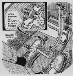
That idle left foot always bothers a veteran driver when he first drives a car that lacks a clutch pedal. Here's one man's solution-an auxiliary horn button on the floor. The switch is a singlepole, single-throw, normally-off job.
