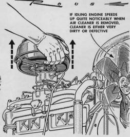
An air cleaner that's dirty outside is undoubtedly dirty inside. So you ought to clean it. Idle the engine as you take it off. If the engine begins to run faster, you can be sure that the cleaner is very dirty—or not functioning properly.
