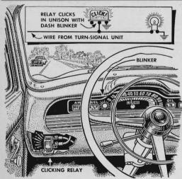
Safeguard against turn signals that continue to blink when they shouldn't by installing this added warning system. Wire a 6-volt DC relay in the circuit with the warning blinker. If you don't see the blinker, you'll hear the relay.
