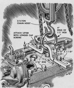
A universal engine lifter is what its developer calls this useful shop accessory. Slots make it possible to attach the lifter to a variety of engines: Merely replace two cap screws with longer screws. The lifter was bent to the desired shape from a bar of %"-by-14" steel stock.
