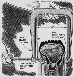
Bead stuck when you start to demount a tire? Here's one way to remove it—if you have or can borrow a deep-throated C clamp of about the dimensions shown. With clamp in place, turn screw to free one side. If the second side remains stuck, use a steel plate as in the drawing.
