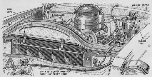
A long pull on a mountain grade may cause an engine to overheat when you are towing a trailer. Spraying the radiator like this will help keep the temperature down. Drill five  $\frac{1}{32}$ " holes in an 18" piece of  $\frac{1}{32}$ " copper tubing. Fasten the tubing to
