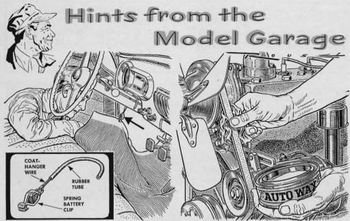
A handy hook like this will keep the floor mat out of the way while a mechanic is servicing a master cylinder that is located underneath the floorboard. The hook will also help to prevent crimping and breaking of the floor mat.
