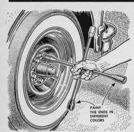
Paint each end of an X-type lug wrench a different color and you'll save all that time that you once wasted looking for the end with the right socket. Just remember the right color for the job you are working on at the moment.
