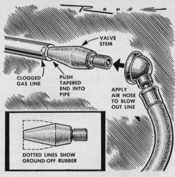
To blow out tubing easily, make yourself a quick-connect adapter that fits the compressed-air hose to lines of almost any size. The adapter is simply a valve stem from an old tire tube with its end ground to a taper as shown in the inset.
