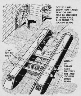
Tightly stuck tire beads are broken effortlessly by one garageman—he lowers the grease rack on them. For most tires, a pair of hardwood two-by-sixes six feet long are placed edgewise across the tire next to the rim. For big tires that just span the rack, no spacers are needed.
