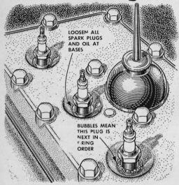
Bubbles in oil reveal the firing order of the cylinders when you have to check the timing of a strange engine. Loosen the spark plugs, squirt a little oil into the spark-plug wells, and then crank the engine slowly while you watch the order in which bubbles appear in the oil.
