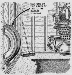
Squeezing a new car into an old garage just about requires wall bumpers. Among the best are sections cut from an old tire. Notch them at each end so that they can be nailed over the studs.
