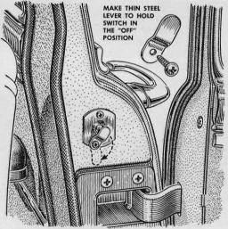
Want interior lights off-with doors open? You can get around the automatic door switches by fastening little levers, bent from thin steel, under the switchmounting screws. Just flip the levers up when you want to hold the switches off.
