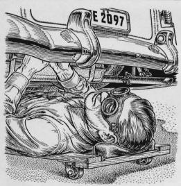
Protect your eyes from falling dirt and dripping grease and oil by wearing goggles when you're working underneath a car. Swimming goggles will do the job nicely and are generally available for less than a dollar a pair.
