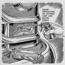
**Squirt penetrating oil** around a tail-light or parking-light bulb that you find rusted fast to its socket shell. Otherwise, you run the chance of damaging the socket. Coat the socket and the new bulb with oil so that removal next time will be fast and easy.
