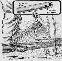
**Dropping a ratchet** onto a cement floor, when the tool is being used with a socket set under a car, is a common occurrence. Often the small lever is snapped off. As a safeguard, one mechanic slipped a piece of rubber hose over the wrench, like this.
