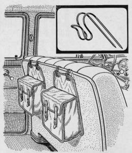
A pair of bicycle saddlebags mounted like this will add a lot of useful storage space to a sedan. The bags look good, too. Form a pair of supporting pins for each bag from 1/16" piano wire and sharpen the points. Just push the pins down into the upholstery. The bags can be lifted off the hooks and used as carriers if desired.
