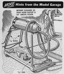
A vacuum cleaner mounted on a rolling stand like this makes it easier to clean car interiors in a service station. Dragging on the floor is eliminated and the cleaner is kept out of grease and dirt. A more effective hose length is achieved since the cleaner is at cushion height and follows easily as the cleaning job progresses.
