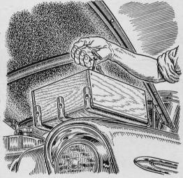
Two-tone parts boxes are not yet a necessity in a service garage. But one operator says that frequent replacement of gritty old boxes with new, clean ones pays off. Soft rubber on the bottoms protects fenders. Parts are cleaned before they're put back.
