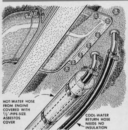
An underseat heater may lose heat from a long supply line. If you have this type of heater, better check to see whether you can do something about insulating the line. Applying the snap-on type of insulation used in houses will do the trick very effectively.
