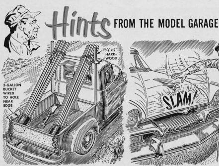
Carrying long pieces of pipe in a pickup truck is easy when you do it this way. Install empty pails in the rear corners of the truck bed to serve as quivers for the ends of the pipe lengths. Be careful if you should come to an underpass that's a bit low.
