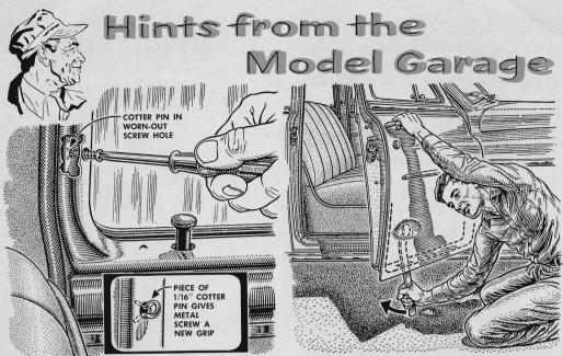
A cotter pin will fix an oversize hole into which molding must be screwed. Spread the pin, squeeze together and put it into the hole. The screw, which is of harder metal than the pin, will force itself between the pin and the side of the hole.
