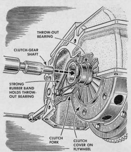
In reassembling a clutch, one mechanic uses a rubber band to keep the throw-out bearing in its yoke while he pushes the transmission clutch-gear shaft through it. Left in place, the band soon breaks and falls out of the way. The idea is especially good for Chevvy clutches but can also be used on some others.
