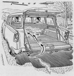
**Exhaust gases** tend to swirl forward into a station wagon when it is driven with the tailgate down. If you must keep it open, remember to open all the windows and ventilators while you drive.
