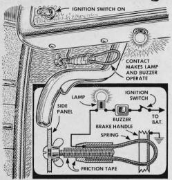
A parking-brake signal will cure the absent-minded who tend to start off with the brake set. A buzzer buzzes and a light stays on until you push the brake handle away from the coil spring, breaking the circuit that is set up when the ignition switch is turned on. Tape insulates the spring from its mounting bolt.
