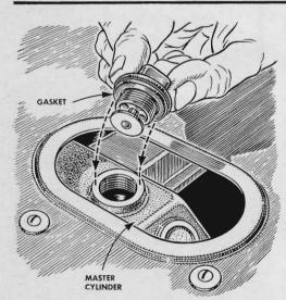
When adding brake fluid to the master cylinder, be sure that there's a gasket under the cap—or it may stick the next time you try to remove it. And don't tighten too hard. Caps sometimes break.
