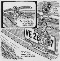
A rear trunk key also serves as a gas-cap key in this setup for a car that has the filler pipe hidden behind a tilt-down license plate. A steel strap projecting from the deck lid prevents access to the gas cap until the lid is lifted.
