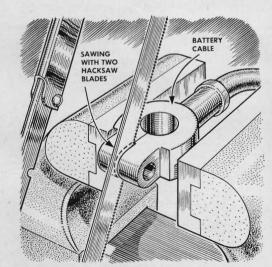
If the hole of a battery clamp is too big to fit snugly on the post, remove the cable from the car, clamp the terminal in a vise, and hacksaw along the lips with two blades. This removes enough metal to fit the clamp to the post.
