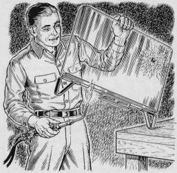
Removing a window channel to replace the glass is often a tough job, especially if rust has formed on the metal. To save time and temper, apply heat to the bottom side of the channel with a torch.
