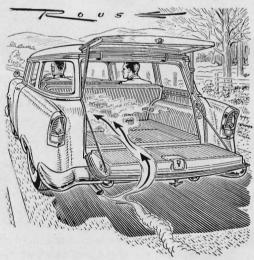
**Exhaust gases** tend to swirl forward into a station wagon when it is driven with the tailgate down. If you must keep it open, remember to open all the windows and ventilators while you drive.
