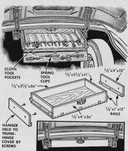
Tools won't rattle or be in the way if they're stowed in a space-saving drawer like this one built to fit between the reardeck hinges. Fasten wood side rails to the hinge covers with self-tapping screws and fit a cupboard catch to the drawer front to keep it from sliding.
