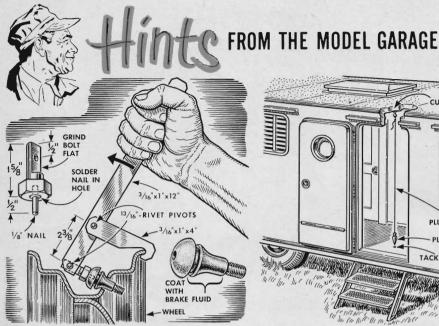
Improvised lever tool, assembled from steel strips, applies straight, firm pressure to insert tubeless valves in wheel holes without damaging them. The hook acts as a fulcrum against the wheel rim, and pressure on the long end of the handle is multiplied at the short end. Application of brake fluid makes insertion easier.
