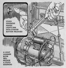
When an engine won't start after slow cranking in cold weather, the starter pinion-gear sometimes stays in mesh with the flywheel gear, holding the contacts together. You can check this by turning on the dash lights before starting. If they remain dim after cranking, tap the solenoid to release the plunger and open the contacts.
