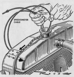
An old speedometer cable, removed from its housing, makes a good flexible snake for cleaning a clogged overflow pipe. This is important maintenance because pressurized cooling systems relieve excess pressure through the overflow pipe.
