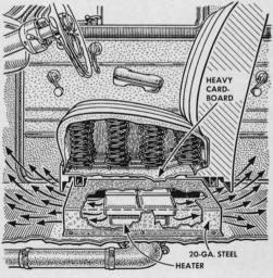
Minimize heat loss this winter by making a sheet-metal duct to fit over an underseat heater. The duct, open at both ends, permits free circulation, yet prevents the heat from rising and accumulating in the spring pocket under the seat.
