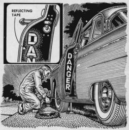
Flash a brilliant warning to oncoming motorists at night by arranging strips of red fluorescent tape to spell out DANGER on the edge of your left front door. It will be visible every time you open the door or make roadside repairs.
