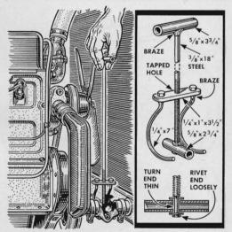
Almost like a mechanical hand, this tool bends a replacement radiator hose and positions it between the lower radiator connections. Unscrewing the handle straightens the hose and it is then nudged over the fittings by hand.
