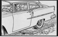
Old rugs can be useful around a car. Instead of throwing them out, cut them up, stow a few pieces in the trunk and leave the rest in the garage. Spread them on the ground or over dirt or mud when making repairs or changing a tire. If you get stuck in snow or mud, toss one under a rear wheel for traction.
