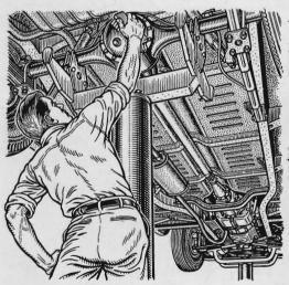
Running gear will run cooler if steamcleaned or brushed with solvent once a year. A coating of grease and dirt on the rear axle, transmission and oil pan keeps the heat in, thinning out the lubricants and reducing their efficiency considerably.
