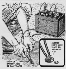
If the terminal marks on a battery are worn, attach two wires to it and hold their ends in a drop of battery acid, salt water or saliva. Move the wires close together and bubbles will form around the one that leads to the battery's negative terminal.
