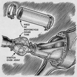
Universal joints will stay free of dirt and mud with these protective covers. Cut pieces about 10" long from a small-size inner tube and have your garageman slip them on the next time you have the bearings packed. Close the tube ends with hose clamps.
